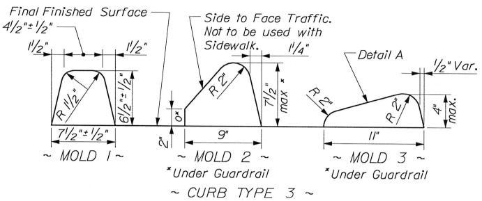
Curb Mold 2 or 3 shall be used in all situations except for where the curb forms the edge of the sidewalk. Mold I shall be used in conjunction with sidewalks or where there is a potential for sidewalks. Mold 3 shall be used in situations where the design speed exceeds 45 mph. Maximum height of Curb under Guardrail shall not exceed 4".
